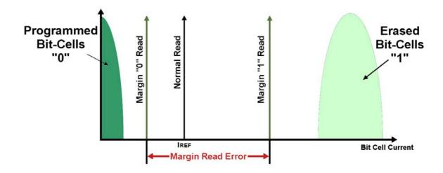
The Verify in normal read mode performed after programming does not catch this failure. This Verify is at the data level and compares the data content of programming file with the data content of the memory space of the device but does not test the quality of the programming.
