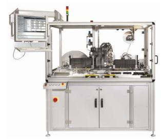
compliment the SmartHandling concept. Every device is vision checked prior to placement in the programming socket. The coplanarity check is performed after programming as an additional safety check. A third vision system monitors device placement at the taping station to ensure after programming a uses automated lead scanning systems to verify that tolerances adhere to manufacturer or customer specifications.
